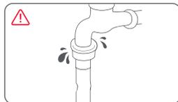
Connect the machine to the tap with a new water inlet hose, and replace the hose in time in case of damage or leakage.
