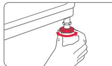
3. Rotate the leveling feet to obtain desired height.
