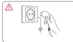
To avoid danger, the damaged power cord of the machine must be replaced by a professional sent by the service department of the manufacturer.
