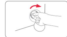
4. Put the filter element back into the drain pump and tighten it, and close the drain pump flap.
