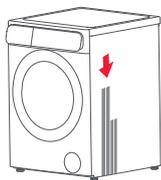
1. Find four noise reduction pads on foam supporting board.
