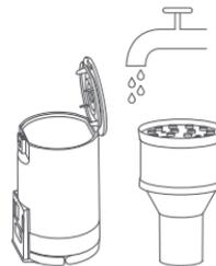
3. Leave the dustbin and cyclone separator to dry for 24 hours or until completely dry.
