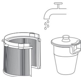
4. Shake off any remaining water and leave the filter to dry for 24 hours or until completely dry.
