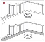
1. Tidy cables and loose items from the ground and move any unstable, fragile, precious, or dangerous items to prevent personal injury or property damage due to items becoming tangled in, struck by, or knocked over by the robot.
