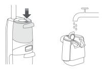
3. Reinstall the Clean Tank bottom first then push forward to secure it in place.
