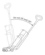
**Caution:** In order to prevent dirty water from leaking out, do not lay the body flat or tilt it over 60° when dirty tank in place.
