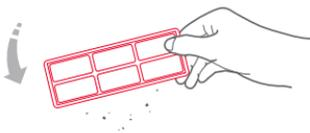
5. Dry the filter thoroughly and reinstall.
