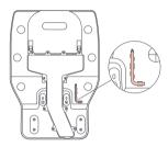
2. Place dock upside down on a soft, flat surface (carpet/towel/ cloth) and attach the base by using the six screws provided.
