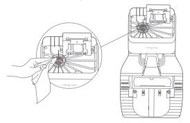
4. Install a new dust bag in place along the slot and put the dustbin cover back.
