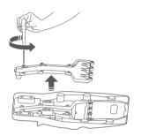
2. Wipe the air duct and cover with a dry cloth.
