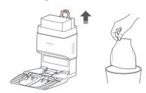
Note: The dust bag handle seals the bag on removal to prevent dust leakage.
