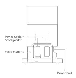
Note: Power cable can be pulled out at both sides.
