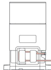
4. Place the dock on a hard and flat floor (wood/tile/concrete etc.). Keep at least 0.5 m (1.6 ft) of clearance on either side, 1.5 m (4.9 ft) in front, and 1 m (3.3 ft) above. Check the location has good WiFi then plug it in.
