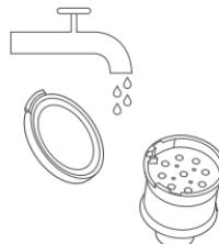
5. Leave 24 hours for the Front Filter and Multi-Cyclone Assembly to dry thoroughly.
