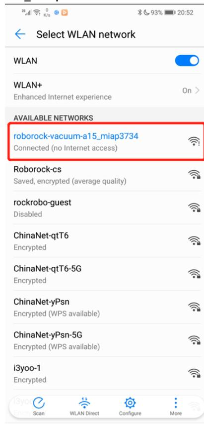
3.10 Once the robot's wifi is selected, the robot will say "connecting to wifi", and the wifi indicator light will flashing rapidly. Then go back to the Mi Home app. Wait until your device connects to the Wi-Fi. The Wi-Fi indicator on the top of your vacuum will go from flashing to solid on, and robot will say "wifi connected" if it has connected successfully.
