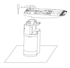
3. Connect the power cable to the dock, and keep excess cable inside the storage slot.
