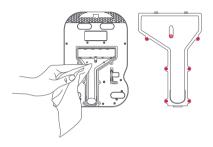
4. Re-install the cover and screw it back in place.
