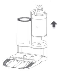
2. Press the Dustbin Opener to open the bottom lid of the dustbin. Rotate the cyclone separator as shown to remove it.
