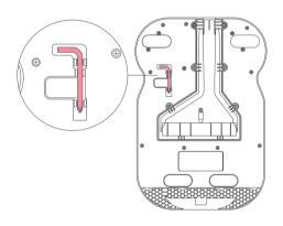
2. Place dock upside down on a soft, flat surface (carpet/towel/ cloth) and attach the base by screwing in five screws in the areas marked with a , as shown.
