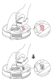
**Note:** Make sure the dustbin provided with the robot has been replaced with the autoempty dustbin or it may fail to empty automatically.
