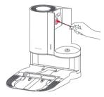
2. Unscrew the screws (7) and remove the cover.
