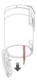
Note: The dust bag handle seals the bag on removal to prevent leakage.
