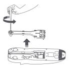
3. Wipe the air duct and cover with a dry cloth.
