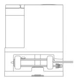
4. Place the dock on a hard and flat floor (wood/tile/concrete etc.). Keep at least 0.5 m (1.6 ft) of clearance on either side, 1.5 m (5 ft) in front, and 1 m (3 ft) above. Check the location has good WiFi then turn on.
